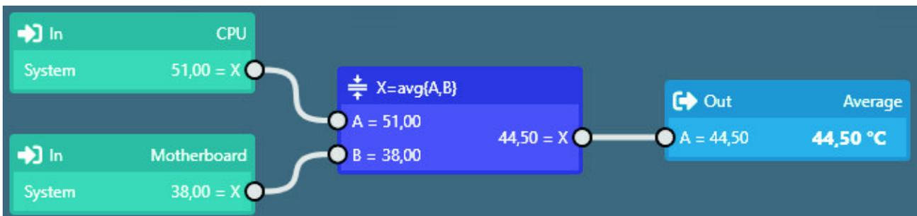
Virtual software sensors are updated once per second and re-calculated with the numbers valid in that particular moment. When using fast changing input values, extreme values can therefore either be used or ignored for the calculation. No smoothing or averaging is taking place.
