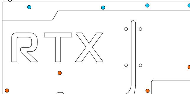
Blue marking: Four screws M2,5 x 8 mm, countersunk head.
