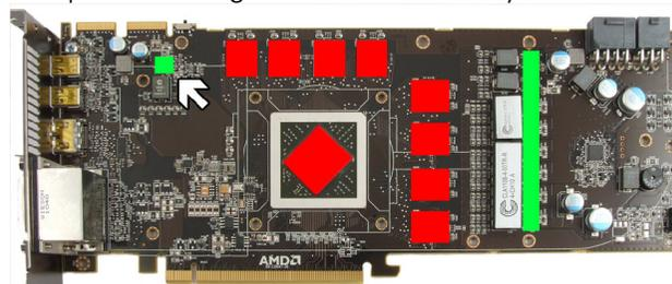
Apply a thin layer of thermal compound to the GPU and the RAM modules (indicated by red marks in the figure). The thermal compound must not be electrically conductive! Cut fitting pieces and place them on top of the voltage regulators (indicated by green marks in the figure).
